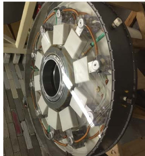
Figure 1 – The prototype BLUE cavity with capacitors and switches installed.
