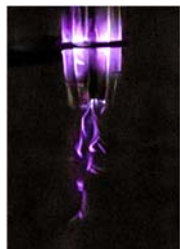
Figure 1: Typical argon plasma jet with filament discharge.
