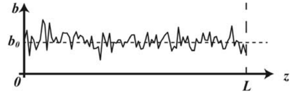
Figure 1 – Example of random variations along tube axis; b is the tuning parameter.
