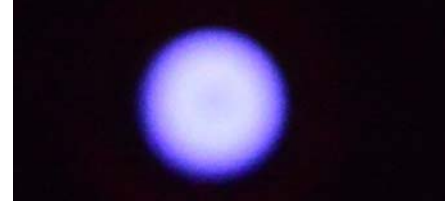
Figure 1 - A front view of the source operating on xenon with \dot{m} = 30 sccm and P_{dep} < 120 W. Note the apparent dim spot in the
