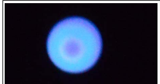
Figure 1 - A front view of the source operating on xenon at \sim 150 W deposited power and 0.5 mg/s. Note the dim center region.
