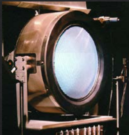
Xenon Ion Thruster (NEXT)
