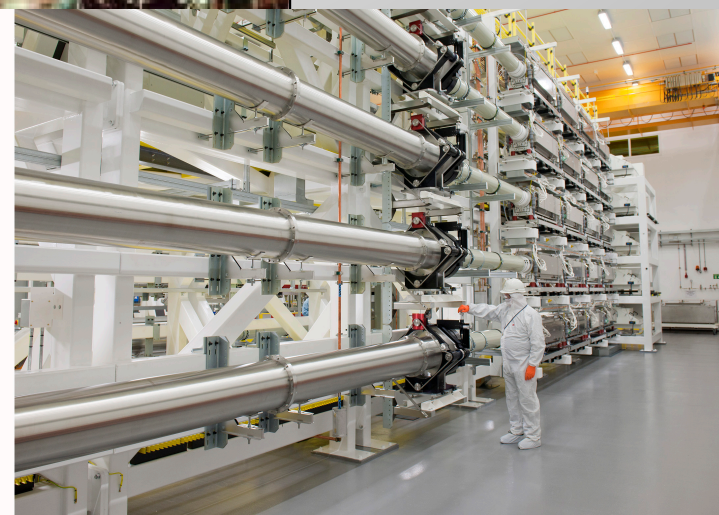
LFEX (ILE) 2-4 beams, 1 ps, ~1 kJ each beam
