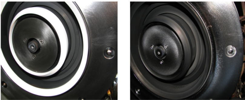
Thruster surface erosion
