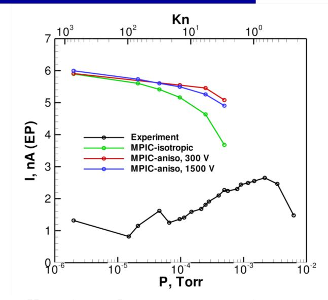
Refined anisotropic model brings IC current collection closer to experiment.
