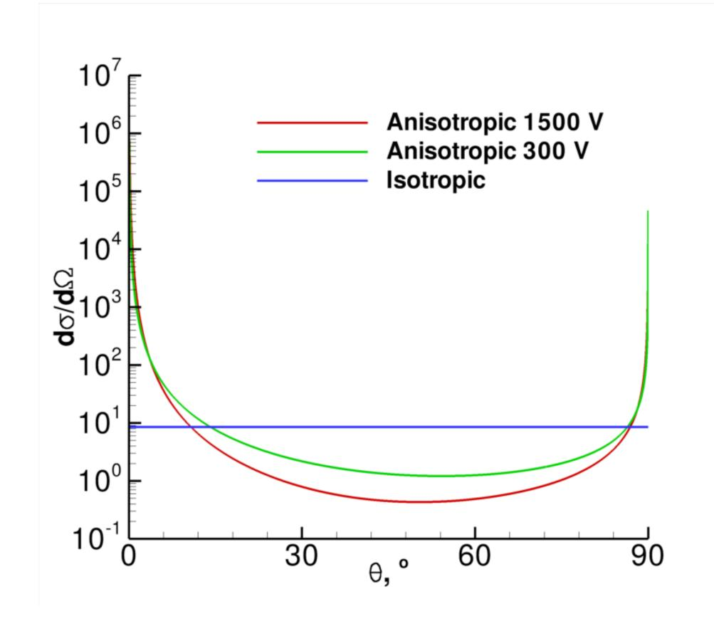
**Isotropic**: Uses total cross-sections of *Miller*, et al. [1], in which a post-collision scattering angle is assigned randomly via a unit-sphere.
