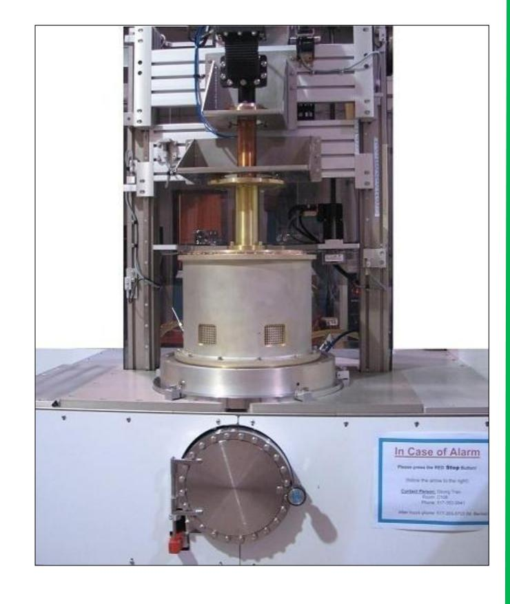
The ECR Microwave Plasma Diamond Etching Reactor Microwave Plasma Assisted Diamond Etching
