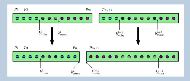
This method can be adapted to multi-cell crossing scenarios such as particle insert, 2D and 3D spacefilling curves. The following diagram shows a hierarchy of bucket sorts that can handle multiple cell crossings following an arbitrary space-filling curve.
