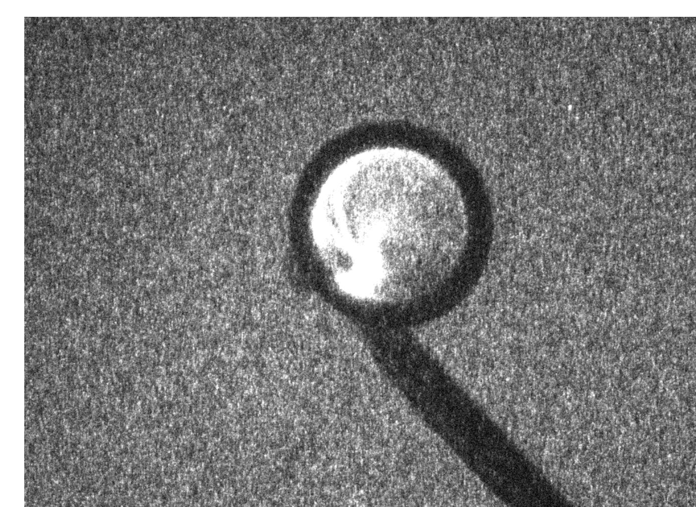
Propagation occurs along the air-water interface due to local electric field enhancement caused by E . [5]
