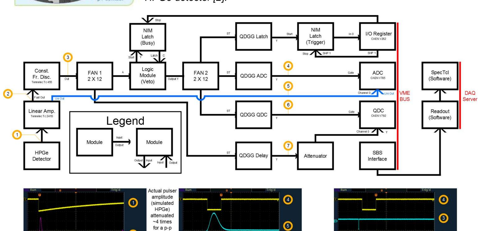
Above: Block diagram of the data acquisition system for the HPGe detector. The blue Gaussian like signal (5) is used to resolve energy by measurement of the peak voltage when the logic gate (4) is true. The initial timing signal (2) is delayed so it occurs coincidentally with (5) and is fed into a charge integrator which can then count how many events arrive when (6) is true.
