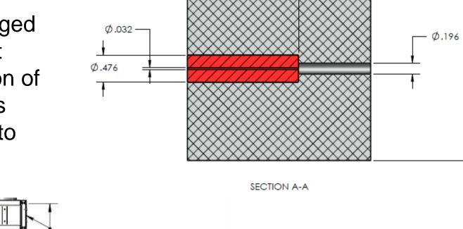
Above: A thick lead collimator cube with cylindrical tungsten insert to reduce the solid angle observed by the detector.
