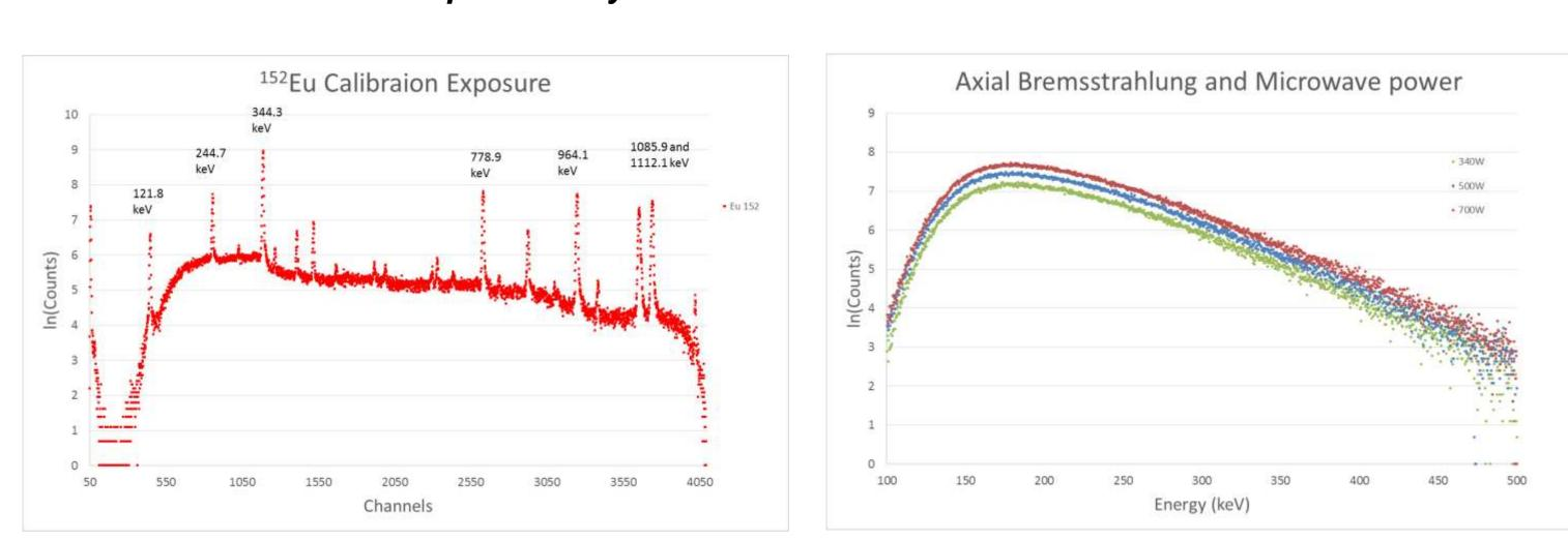
On Left: Europium 152 with distinct spectral lines that allow for calibration of channels to energies. On Right: Bremsstrahlung as measured from SuSI for three different microwave powers. For each setting the slope and terminal energy of approximately 475 keV do not change significantly.
