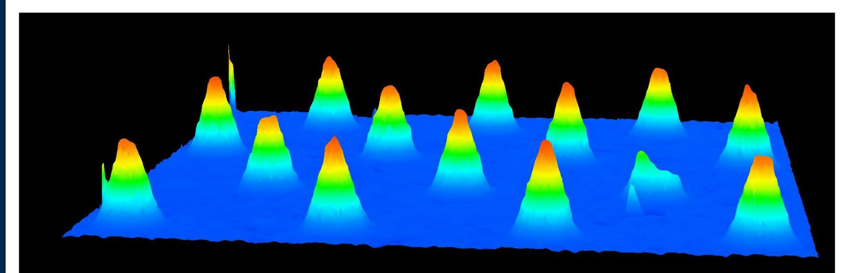
Through surface profilometry and geometric modeling, we can measure variability (tolerances) in the emitters.
