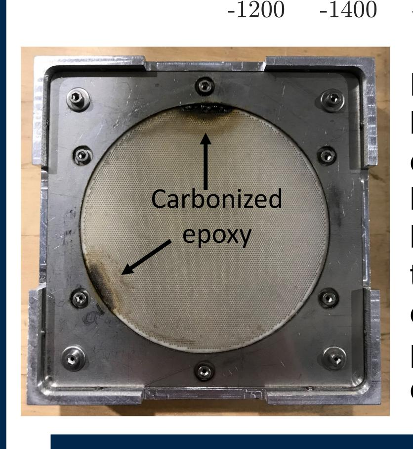
Extended manufacturing to make 25 W class emitter chip (>10,000 emitters) in 3 hours machine time Bow in extractor limited thruster to 3.4 W over throttle
