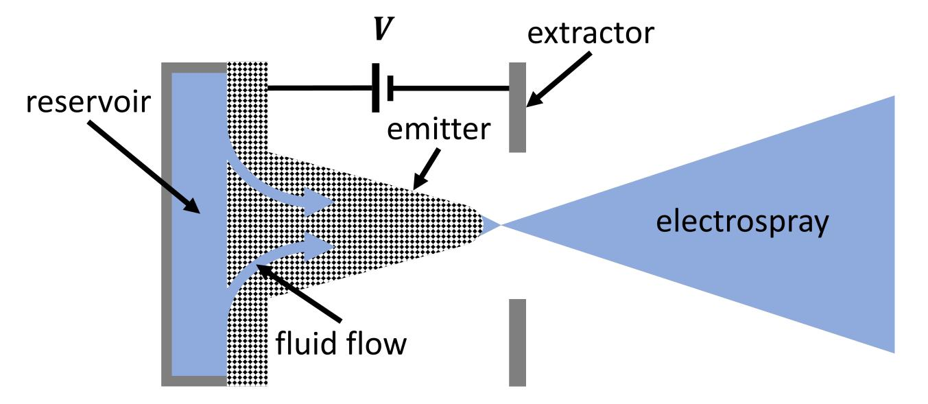
This technology is well poised for smallsat scale electric propulsion, where heritage EP systems (Hall & ion thrusters) suffer performance losses. However, individual emitters operate at the microscale, so many must be aggregated together to increase power. While SOA has achieved arrays of hundreds of emitters, this still lags demand:
