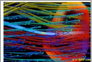
Field lines associated with flux ropes. Magnetic field lines (red, green tubes), plasma current (arrows) and the QSL. [Phys. Rev. Lett., **103**, 105002 (2009)]
