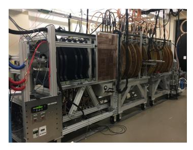
The PHAse Space Mapping (PHASMA) experiment at WVU; measures distribution functions of both ions and electrons in a space-relevant plasma (e.g., Shi et al., Phys. Rev. Lett., 128, 025002, 2022)
