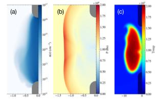
Plasma-assisted ignition in an ethylene/air mixture: (a) plasma discharge (0-100 ns); (b) acoustic expansion (100 ns - 5 us); (c) kernel ignition and outward flame propagation (5 us to 10 ms).
