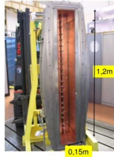
CYBELE negative ion source for NBI under development @ CEA Cadarache
