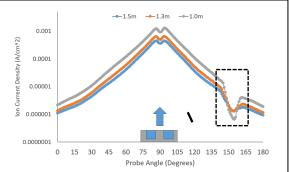
Figure 1 - Plot showing the effects of the carbon shield on the measured ion current density at three different radial distances.
