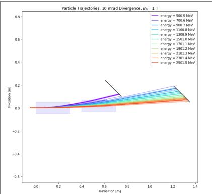
Figure 1-A general setup of the magnetic spectrometer simulation using an analytic block-dipole magnetic field regions of dimensions of length 0.3 m, width 0.1 m, height 3 cm, and central field strength of 1 T, as well as particle trajectories of various energies on axis and 10 mrad divergence on the y-axis landing on two catching screens. Energy resolution of this setup as measured by deflection by the magnetic system on the catching screens.
