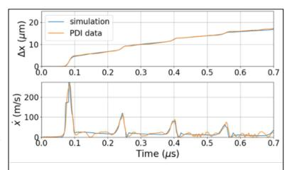
Figure 1 - Simulated tracer particle trajectories vs. PDI data from experiments with Ti-6Al-4V exposed to a Xenon source
