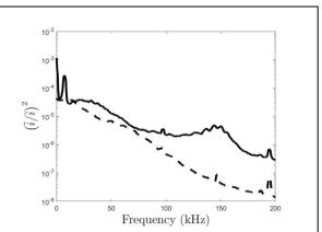
Figure 1 – Power spectrum of waves in the plume of a magnetic nozzle for a low (solid) and high (dashed) flow condition. The high Flow dampens all modes, but the low Flow maintains distinct peaks at 10 kHz, 40 kHz, and 100 kHz.
