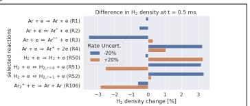
Figure 1 – Sensitivity analysis of  $H_2$  density:  $H_2$  density change after 10 pulses (t=0.5 ms) due to  $\pm 20\%$  change of reaction rate coefficient of selected reactions in nanosecond pulse discharge in 1%  $H_2$  - 0.15%  $O_2$  - Ar mixture.
