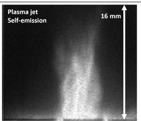
Figure 1 – Self-emission image of the aluminum plasma jet at 216 ns after pulse start. The jet is traveling at around 100 km/s and has an estimated density and temperature of  $10^{-4}$  g/cc and 20 eV respectively.
