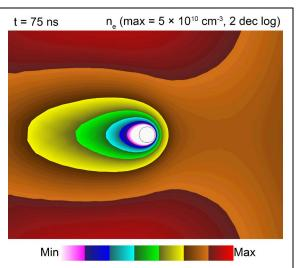
Figure 1 – Electron density at 75 ns from the start of the 40th RF cycle. The dielectric droplet is 40 microns in diameter and nonconductive, with an RF voltage amplitude of 200 V.
