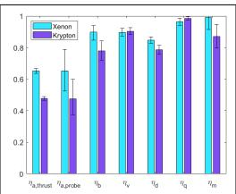
Figure 1 – Efficiency contributions for the H9 running on xenon and krypton at 300 V, 15 A.
