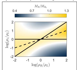
Figure 1 – The shock strengthening, i.e. the ratio of the shock Mach number in the experimental target with and without an intermediate density step, versus the overall interface density ratio and the density of a single intermediate step.
