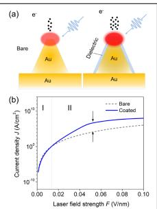
Figure 1 - (a) Schematic of the resonant photoemission from either bare or dielectric-coated Au-nanopyramid field emitters. (b) the photoemission current density J as a function of the laser field strength F, for the bare or coated photoemitters.
