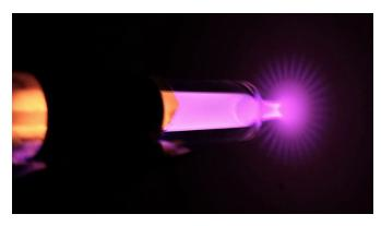
Helium Atmospheric pressure plasma jet "blooming" towards the surface of a thick glass-ceramic block (macor). 1 slm helium flow, -10kV, 2us DC square pulse width, 10 mm tube-outlet glass-ceramic distance.
