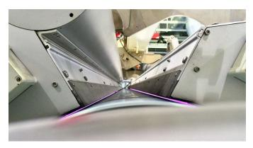
This image shows 2 electrodes, 8.72 m long, discharging with 96 kW each against an isolated roller (DBD) in ambient air, used in a BOPP production plant, Source: SOFTAL Corona & Plasma GmbH, Germany. **Dr. Florian Brehmer**, Brehmer@AFS.biz, www.afs.biz.
