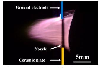
A low temperature air plasma jet based on a rotating electrode. The device can be used for surface treatment, plasma chemistry, plasma medicine applications and studying the mechanism of air glow discharges. Z. Li, J. Liu, X. Lu, Plasma Sources Sci. Technol. 29, 045015 (2020). **Prof. XinPei Lu**, **HuaZhong**, University of Sci. & Tech. <a href="mailto:luxinpei@hust.edu.cn">luxinpei@hust.edu.cn</a>, <a href="mailto:luxinpei@hotmail.com">luxinpei@hotmail.com</a>.
