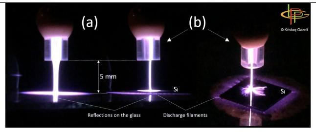
Emission patterns of a ns-pulsed Ar plasma jet impinging (a) on a grounded glass plate and (b) on a silicon (Si) wafer placed on top of a grounded glass plate.
