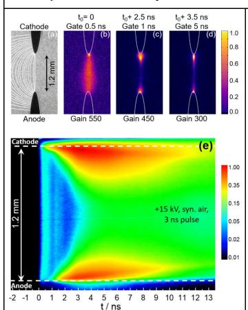
(top) (left) Electrode shape and position overlaid with calculated electric field lines. (right) Single shots of discharge emission structures during initial and secondary breakdown phase, and major emission of 15 kV pulse with 200 ps rise time. (bottom) Spatio-temporal development of the discharge emission along the gap axis obtained by a streak camera in a 15 ns time window in logarithmic intensity scale (accumulation of 100 jitter-corrected streak camera single shots).
