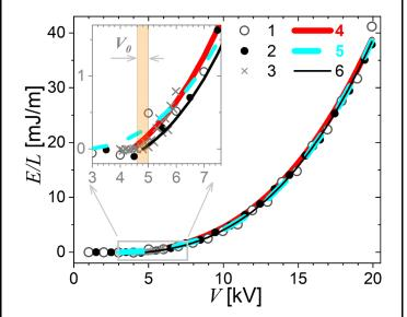
The dependence of the dissipated energy (E) normalized by electrode width (L) as a function of the peak-to-peak amplitude of the applied voltage (V). Points are the measurements, lines are fits using different approximations.
