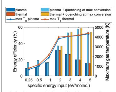
Calculated energy efficiency for CO<sub>2</sub> conversion, as function of SEI, for both plasma and thermal conversion, and the effect of quenching. The corresponding maximum gas temperature is also plotted (right y-axis).
