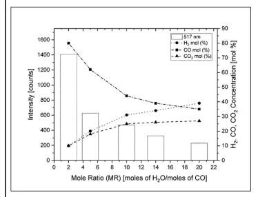
The plasma  $C_2$  (Swan band in nm) vibrational band intensity (primary axis) and the gas composition (secondary axis) versus the MR at 1300 ms of gas residence time and 70 W of plasma power.
