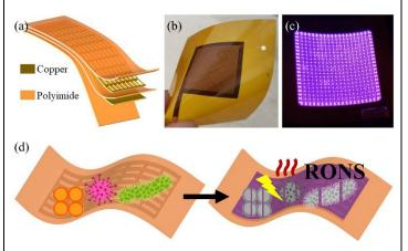
(a) A schematic diagram of the structure of the flexible plasma film; photograph of the film (b) without discharge and (c) with discharge. (d) Schematic diagram of possible disinfection mechanism of flexible plasma film.
