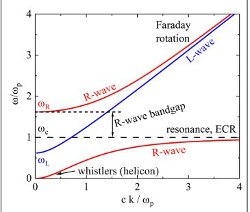
Dispersion relation for the R- and L-waves for the case  $\omega_c = \omega_p$ . The cutoff and resonance frequencies are also indicated. The region of RF frequencies is usually below  $\omega_L$ .
